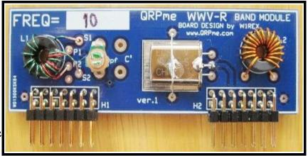
For a 5Mhz band module, the values for T1 are a 15 turn secondary still with a 3 turn primary link. The L2 toroid has 17 turns for 15uh.
