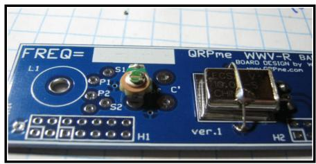
Solder on the two header connectors...
